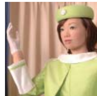
Commissioned by NEDO, the reception robot “Actroid” is equipped with Advanced Media's speech recognition engine (jointly developed with KOKORO CO., Ltd.).
